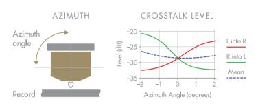
The E Series cartridges use a specially designed adjustment screw to locate the cantilever, rather than the standard fixed pin, allowing micro-adjustments during production. This pre-set azimuth means crosstalk is already optimized and the cartridge can be safely installed in a typical turntable with no correction required.
