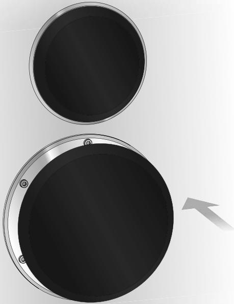
2. Turn it clockwise or counter-clockwise until you can feel the magnets attach to the screws below.
